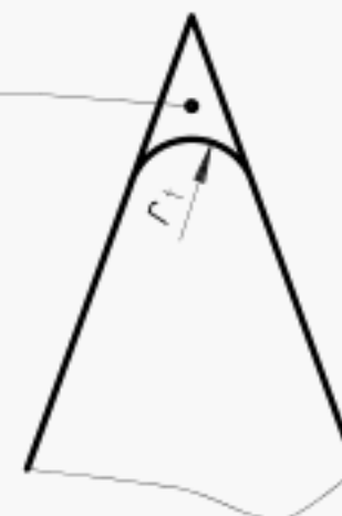
Figure 4 — Cross-section of belt
