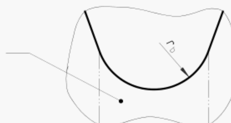
Figure 1 — Cross-section of pulley grooves
