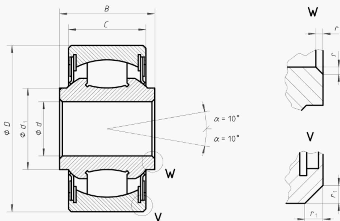
NOTE — The angle of tilt,  $\alpha$ , is a minimum for manufacturers and a maximum for users.
